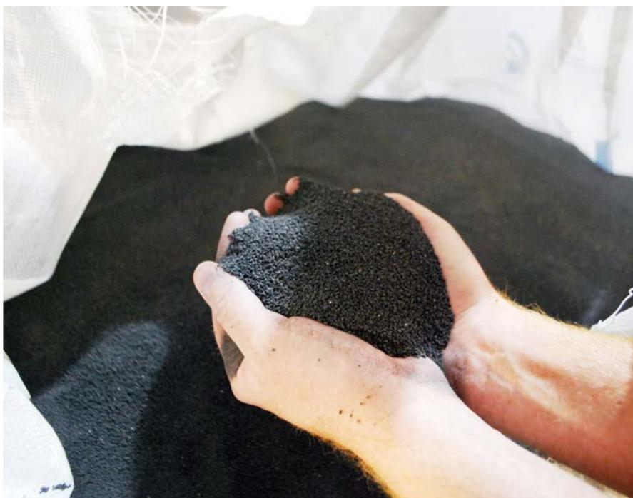
With its large surface area, Filtralite®, an expanded clay media, provides an optimal environment for naturally occurring bacteria that oxidize contaminants during filtration.
