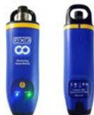
spot GPS coordinates and barometric pressure are viewed through the newest KorEXO software running on both laptops and tablets. The device is IP-67 rated and rugged enough to withstand any drops, drips, or dunks!
