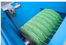
three zones of solids removal to effectively filter high solids waste streams without the use of chemicals. This system is designed to handle a wide range of flows in a fraction of the space compared to conventional clarifiers.
