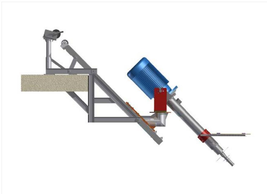
*The sliding pedestal travels on a 45-degree track that allows the aerator to be positioned at the desired height. A pivoting tube allows the aerator to point in any direction.*
