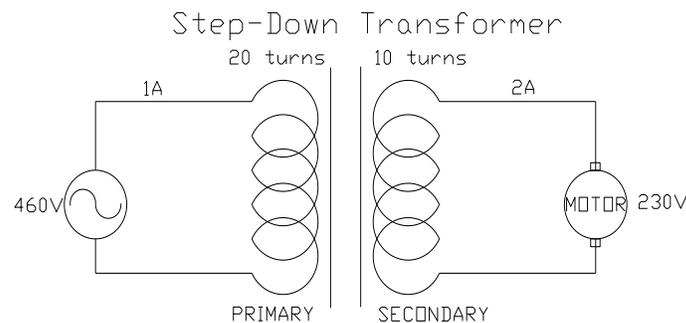
Below are the relationships between the Voltage, Current, and the Turns of a transformer.
