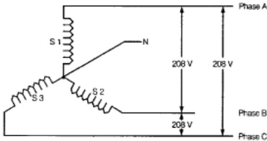
As you can see the Phase Voltage is measured from Phase A to Phase B or Phase A to Phase C or Phase B to Phase C.
