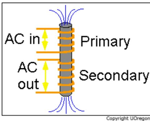
Figure 1-9 show a one to one turns ratio transformer. This transformer has 115V on the primary and 115V on the secondary the primary current is 1 amp and the secondary current is 1 amp. This is because there are the same amount of winding on the primary and the secondary.
