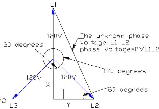
Note: The sum of all angle in a right angle triangle is equal to 180 degrees
