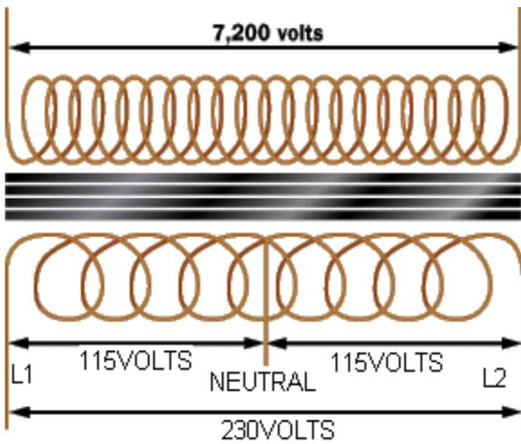
It is important to know that the voltage on L1 and L2 add together, if you were to measure the **phase voltage** you would measure 230V, similarly measuring **line voltage** you would measure 115V. This is because the voltages are 180 degrees out of phase with each other, and their vector sums are additive. Figure 1-3A shows this 180-degree vector relationship.
