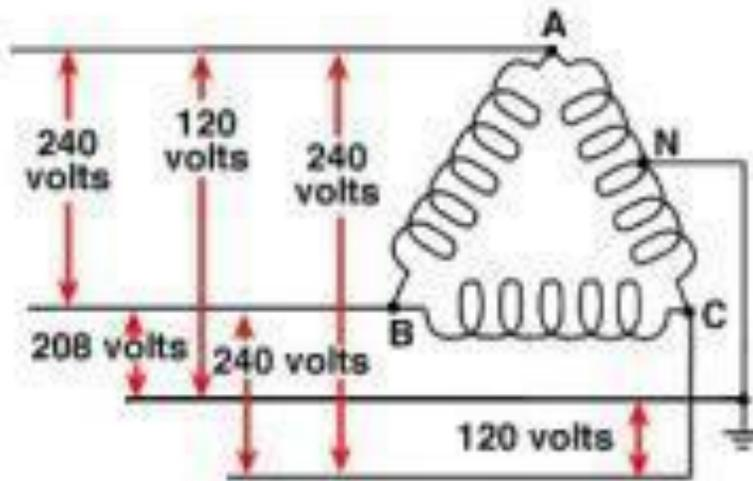
Figure 1-6 Calculating the High Leg Voltage in a High Leg Delta Configuration:
