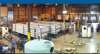
ON THE SHOP FLOOR: Newterra designed, fabricated and commissioned this 12 MLD water treatment plant to treat groundwater for boiler feed at a large steel mill. The system consisted of multi-media pretreatment vessels plus Reverse Osmosis modules. The customer needed a plug and play prefabricated system due to the remote nature of the facility.
